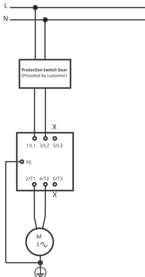
For single phase operation the mode of the soft start must be set correctly in the Advanced menu:
